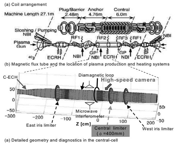
Fig.1 Schematic of GAMMA 10 and camera location
