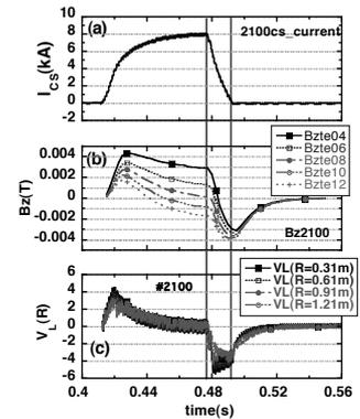
Fig.2. Measured vertical field inside the vacuum chamber for  $I_{CS}=8$  kA. (#2100)
