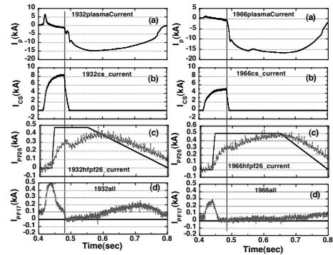
Fig. 1. Plasma current evolution in QUEST at  $B_t=0.14$  T with the one turn cancellation coil. Left column shows  $I_{CS}=8$  kA (#1932) and right one  $I_{CS}=5$  kA (#1966). (a) Plasma current, (b) CS current, (c) PF26 vertical shaping coil current ( $N_{PF26}=72$  turns) and set value, (d) PF17 vertical field coil current.
