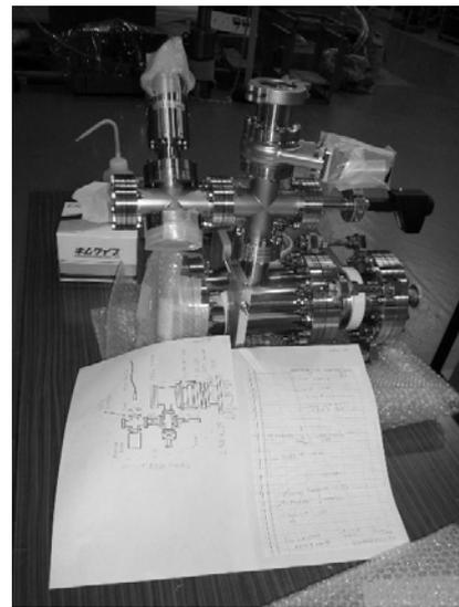
Fig. 21 Snap shot of the vacuum leak test in the Plasma Diagnostic Laboratories
