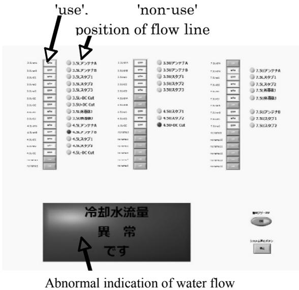
Fig.14 Indication of the warning in the new display system
