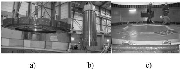
Fig. 17 a) a rotor part of 30 tons b) the rotor shaft c) base of MG
