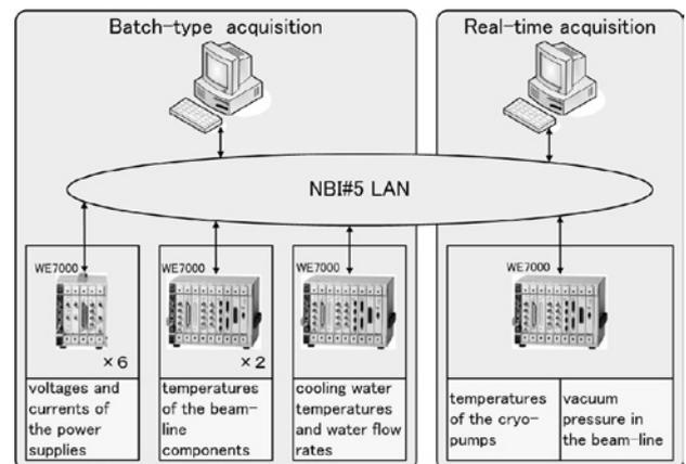
Fig. 16 A schematic diagram for the data acquisition system of NBI#5.
