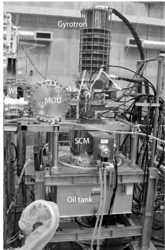
Fig.10 A new 77GHz/1.5MW gyrotron system
