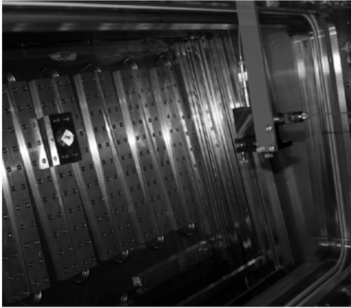
Fig. 19 The optical system to measure transmittance of diagnostics window and cover-glass.
