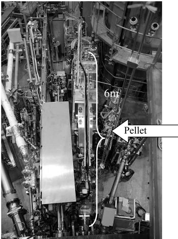
Fig. 5 Twenty-barrel solid hydrogen pellet injector.
