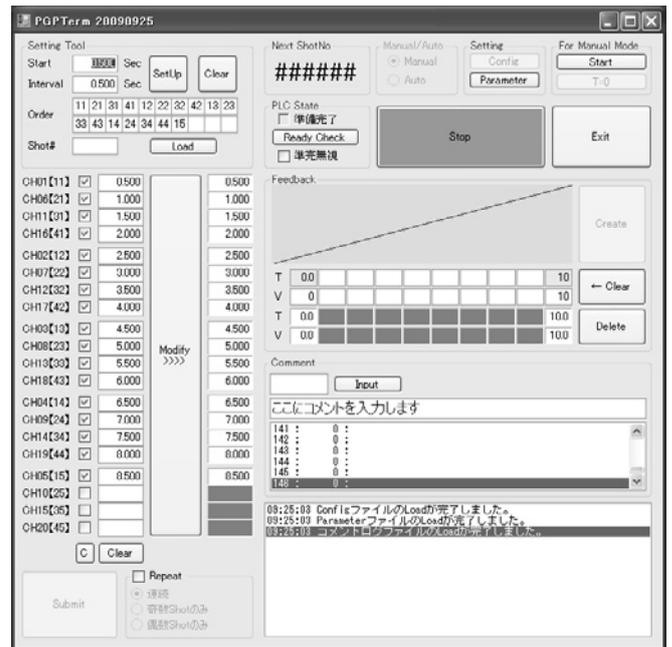
Fig. 26 GUI to setup injection timings
