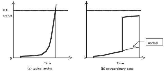
Fig.15 Over-current waveform in arc discharge
