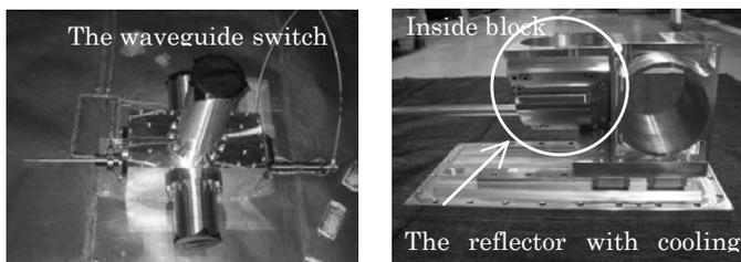
Fig.11 The left photo is the whole outside view. The right photo is the inside moving combination block with the water-cooled reflector.
