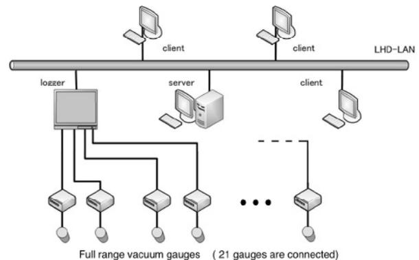
Fig.12. Configuration of a vacuum level monitor system.
