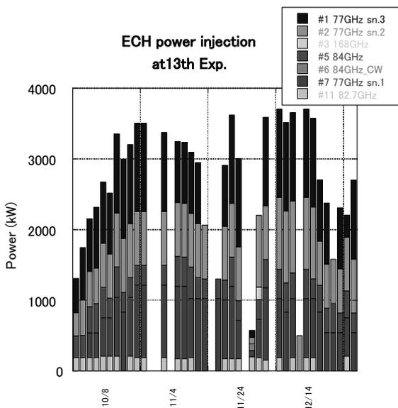
Fig.9. History of ECH injection power during 13th experimental campaign.
