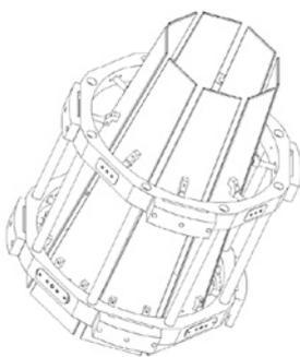
Fig. 20 Design of the new exit side sweeper electrode.
