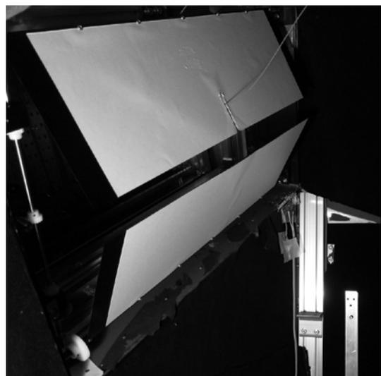
Fig. 18 the light intensity reduction plates.
