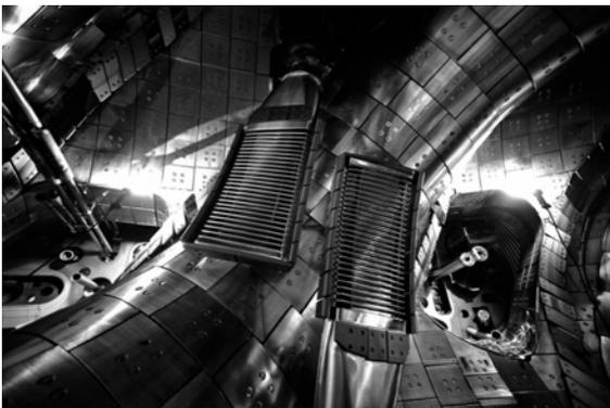
Fig.3 ICRF antennas newly installed on the outboard side of the vacuum vessel. Faraday shields reflect the trajectory of the magnetic field lines.
