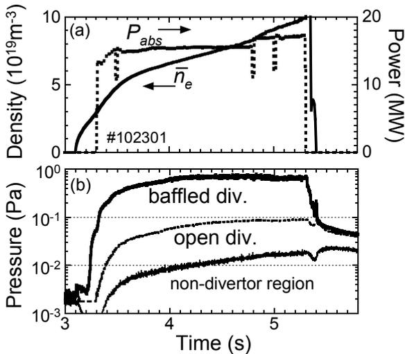
Fig.2 Waveforms of a typical gas-fuelled discharge. (a) Line averaged density and absorbed heating power. (b) Neutral pressures at different locations with regard to the divertor geometry.
