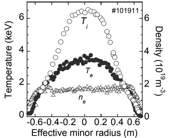
Fig.1 Profiles of ion and electron temperatures and electron density in the discharge with the highest central ion temperature. The signs of the effective minor radius  $a_{eff}$  denotes the inboard side (-) and the outboard side (+) with respect to the center.
