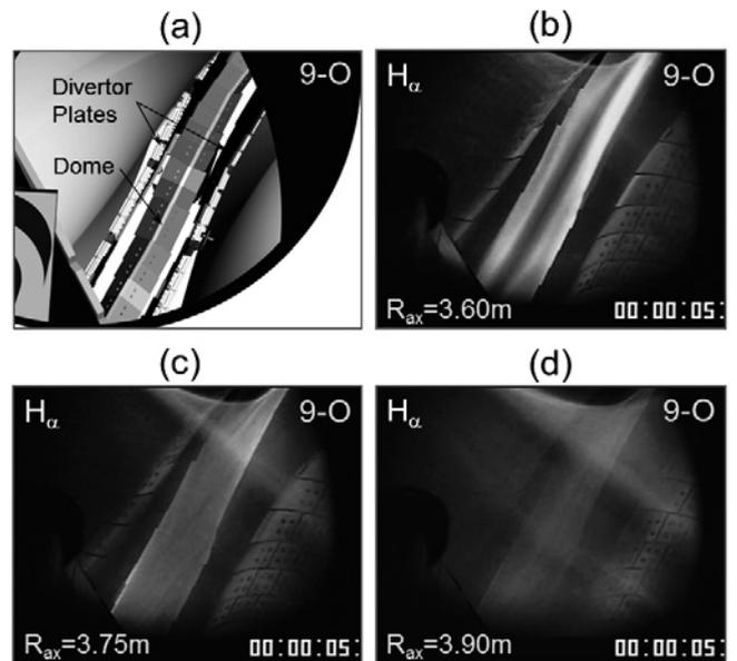
Fig. 1 A CAD image of the CHD configuration installed in an inboard side of the torus (9-I) viewed from an outer port (9-O) (a), a measurement of the image of the intensity of H-alpha emission observed with a filtered CCD camera which is installed in an outer port (9-O) for  $R_{ax}=3.60m$ ,  $3.75m$  and  $3.90m$ , respectively (b), (c) and (d).
