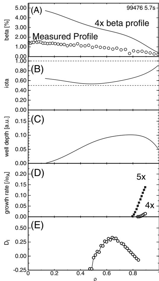
Fig. 2: The measured beta profile (circles) and the assumed profile which is multiplied by four (solid line) (A), the iota profile (B), the well depth(C), the growth rate of the ballooning mode with 4 times(open circle) and 5 times (closed square) case (D) and the mercier condition  $D_I$  (E) are shown.
