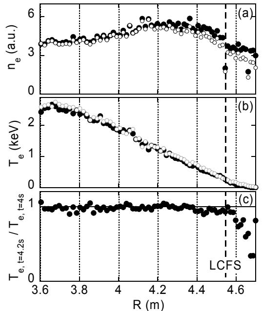
Fig. 2. Radial profiles of (a) electron density ( $n_e$ ), (b)  $T_e$  before ( $t = 4$  s, ●) and after ( $t = 4.2$  s, ○) Ne seeding, respectively, and (c)  $T_e$  ratio between after and before Ne seeding in the same discharge as Fig. 1.
