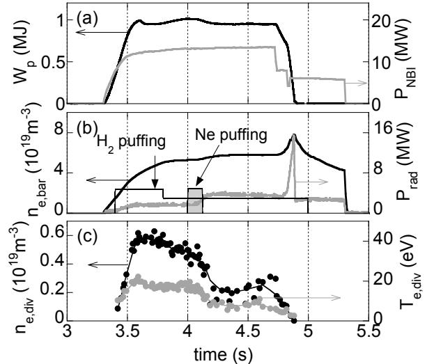
Fig. 1. Typical time evolutions of (a) plasma stored energy ( $W_p$ ) and NBI power ( $P_{\text{NBI}}$ ), (b) line averaged density ( $n_{e,\text{bar}}$ ), radiation power ( $P_{\text{rad}}$ ) and gas-puffing, (c) electron density ( $n_{e,\text{div}}$ ) and temperature ( $T_{e,\text{div}}$ ) in the divertor (torus inboard-side). (#103833,  $R_{\text{ax}}=3.60\text{m}$ ,  $B_t=-2.8\text{T}$ ,  $\gamma=1.2538$ ,  $B_q=100\%$ )
