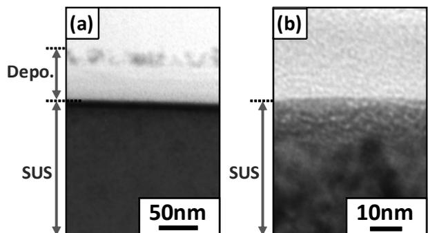
Fig. 3. Cross-sectional TEM image of ground SUS316L specimens at (a) No.1 and (b) No.3 toroidal section.
