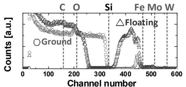
Fig. 1. RBS spectra of ground and floating Si specimens at No.1 section.
