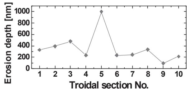
Fig. 2. Erosion depth of the SUS316L ground specimens at each toroidal section.
