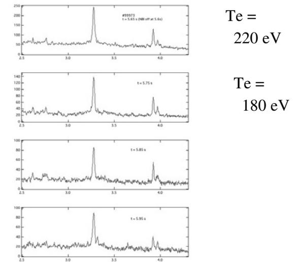
Fig. 2.. The spectrum of carbon ions for non radiation collapse after the NBI heating off.
