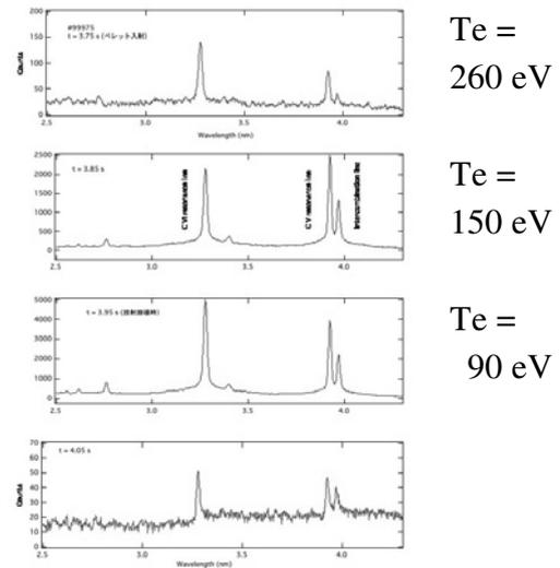
Fig. 1. The spectrum of H-like and He-like carbon ions during the radiation collapse. Te values indicate the temperatures in plasma where  $C^{4+}$  ions exist.
