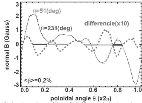
Fig. 1. Calculated profile of differential signals of loops in the plasma with  $m=2/n=1$  magnetic island.
