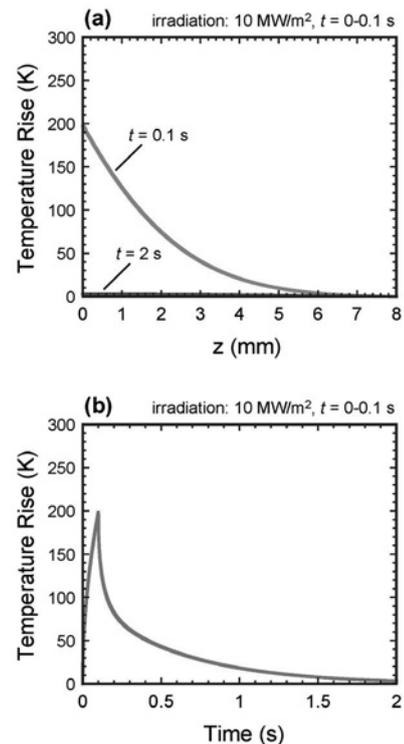
Fig. 2 (a) Temperature distribution in a tungsten slab at times of  $t = 0.1$  and 2 s with a heat flux of 10 MW/m<sup>2</sup> applied to the  $z = 0$  mm surface during  $t = 0-0.1$  s. (b) Temperature rise as a function of time at  $z = 0$  mm.
