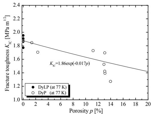
Fig. 3. Relationship between fracture toughness  $K_{IC}$  and porosity  $p$ <sup>3)</sup>.
