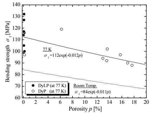
Fig. 2. Relationship between bending strength  $\sigma_f$  and porosity  $p$ <sup>1,2)</sup>.
