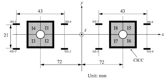
Fig. 2. Cross-section of the conductors near the joint.
