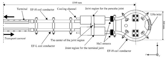
Fig. 1. Schematic view of the joint sample.
