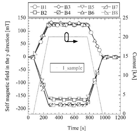
Fig. 3. Measurement results of the self magnetic field without the external magnetic field.
