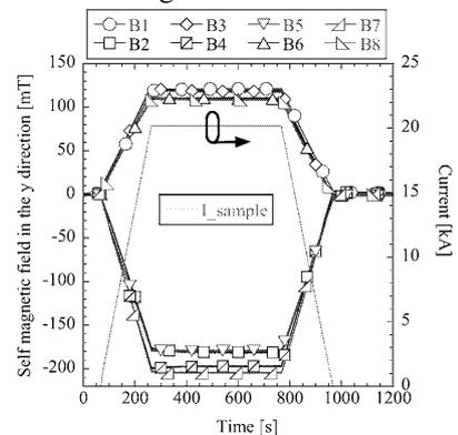
Fig. 4. Measurement results of the self magnetic field under the external magnetic field of 3T.
