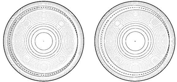
Fig.2 : Contours of helical magnetic flux for  $\Psi_b = 2.0 \times 10^{-3}$  in the initial (left) and the saturation (right) states.
