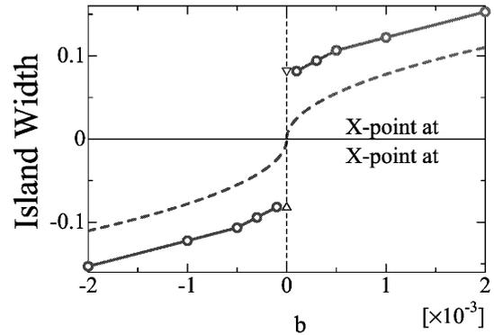
Fig.1 : Dependence of island width on  $\Psi_b$  in the initial (dashed line) and the saturation ( $\Delta$  and  $\circ$ ) states.
