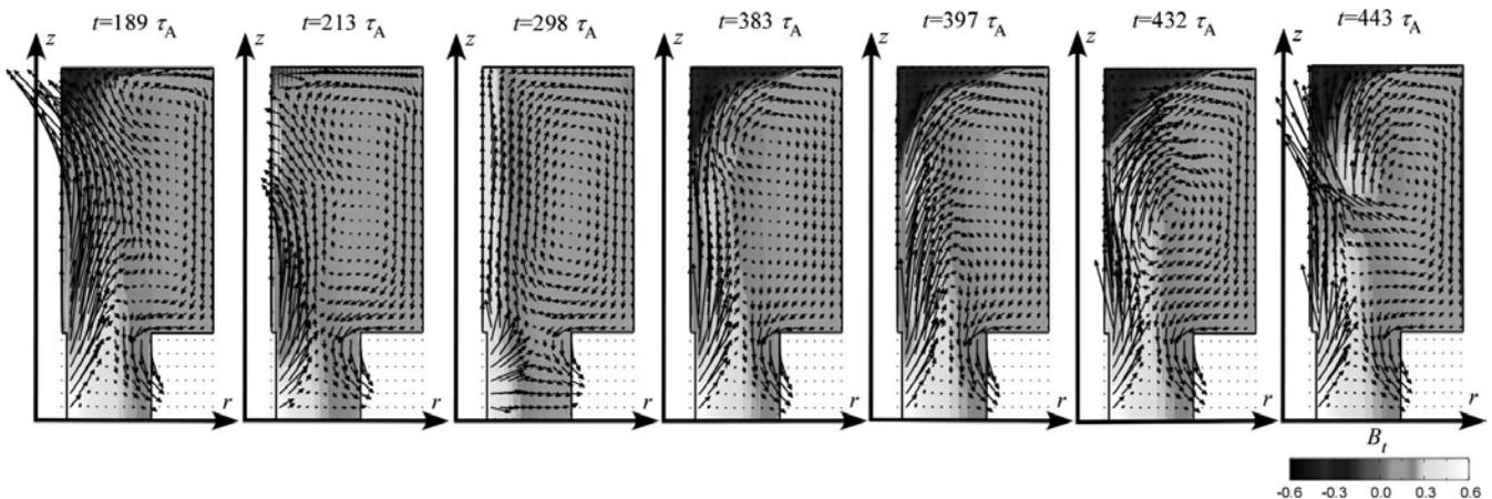
Fig. 1. Time evolution of vector plots of poloidal field  $B_p$  and contours of toroidal field  $B_t$  on the poloidal cross section.
