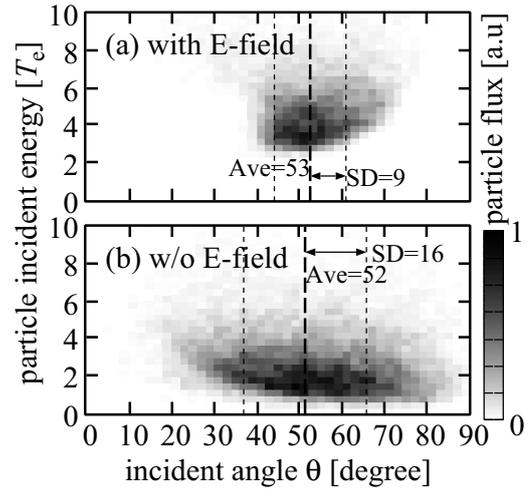
Fig. 1: Contour plot of the particle flux in the case of magnetized plasma for (a) with and (b) without electric field. The averaged angle and the standard deviation of the flux are shown as Ave and SD in the figure. The magnetic field angle is  $\theta = 83^\circ$ .
