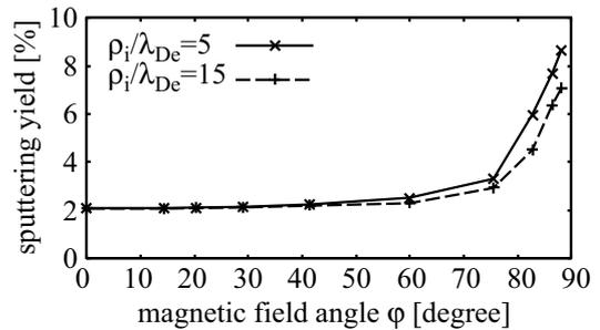
Fig. 2: Physical sputtering yield calculated by the Bohdansky-Yamamura model from the PIC simulation results; dependences on  $\rho_i/\lambda_{De}$ .
