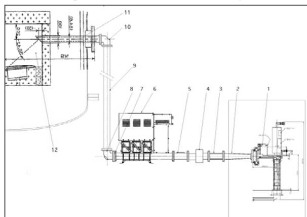
crystron microwave generator① to applicator⑫, water-cooled isolator④, directional coupler⑤ and 3-stab auto tuner⑥ were connected.
