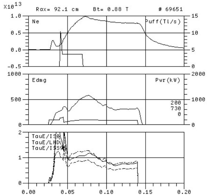
Fig. 2. NBI discharge with deuterium gas puff
