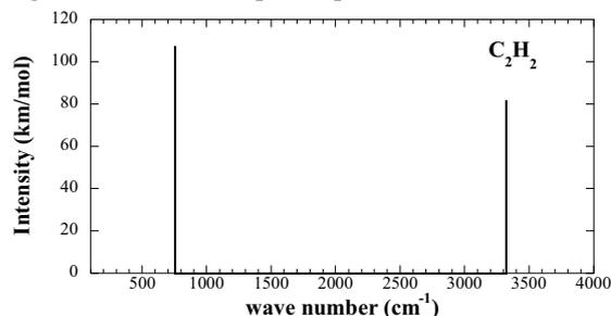
Fig.2 Infrared absorption spectra calculated with Gaussian 03 for C<sub>2</sub>H<sub>2</sub>.
