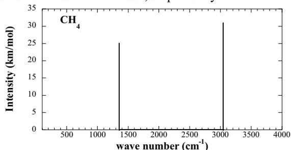
Fig.1 Infrared absorption spectra Calculated with Gaussian 03 for CH<sub>4</sub>.
