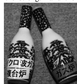
Fig. 1 Bright coloration of Gosu Left; microwave gas hybrid kiln Right ; gas kiln
