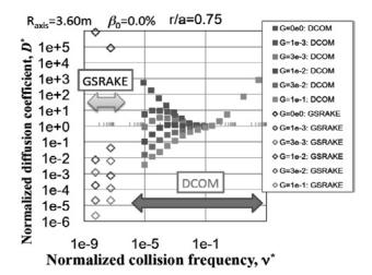
$v^{*} = \frac{Rv}{\iota v} \qquad G = \frac{R_0}{\iota r} \frac{E_r}{v B} \quad D^{*} = \frac{D}{D_{Plateau}} = \frac{\iota \pi R_0}{0.64 \rho^2 v} D^{*}$
