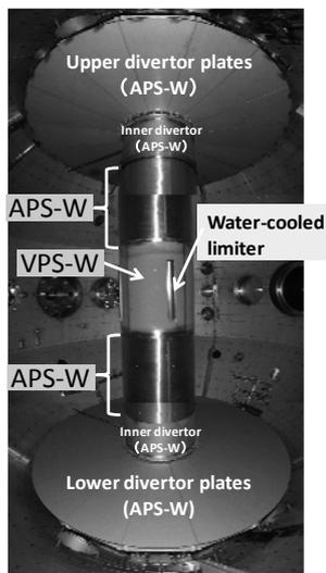
Fig. 1 Internal view of the vacuum vessel of QUEST.
