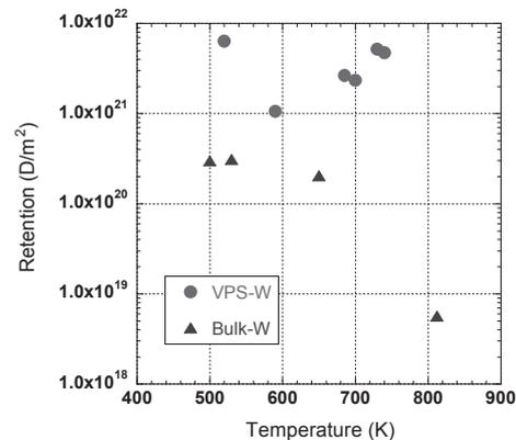
Fig.4 Surface temperature dependence of deuterium retention of samples of VPS-W and bulk-W.
