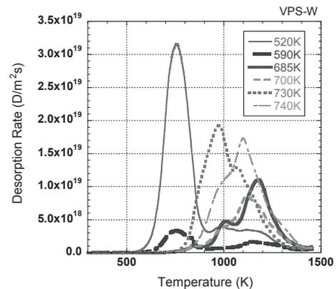
Fig.3 TDS spectra of VPS-W samples of which surface temperature during plasma exposure is in the range of  $520 \text{ K}$  to  $740 \text{ K}$ .
