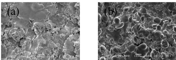
Fig.2 SEM micrographs of (a) APS-W and (b) VPS-W.
