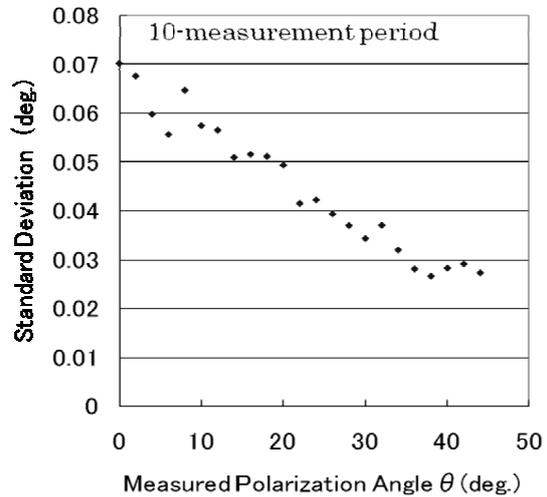
Fig. 2 Polarization angle dependence of the measurement errors with the dual PEM polarimeter.
