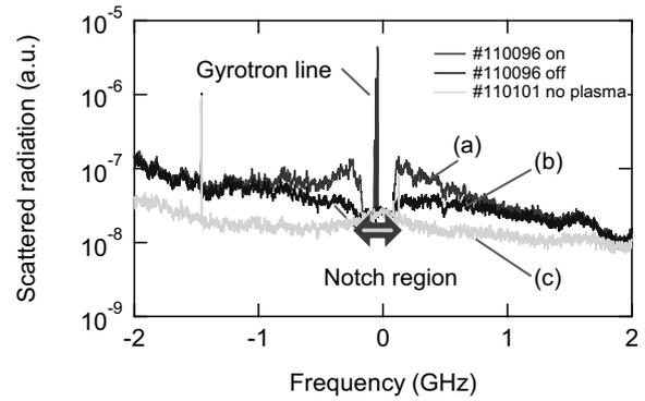
Fig. 2. Measured spectra for (a) probing beam on, (b) probing beam off, (c) system noise.
