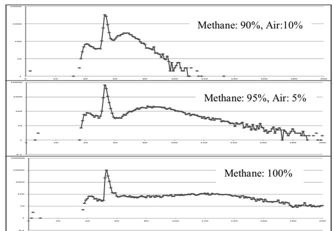
Fig.2 Effects of air condition on rise time spectrum.
