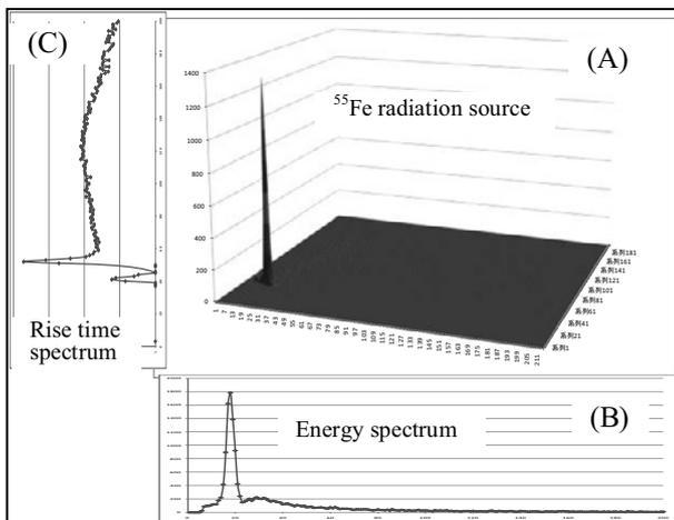
Fig.1 Two-parameter-spectrum of  $^{55}\text{Fe}$  of a proportional counter filled with pure methane gas.
