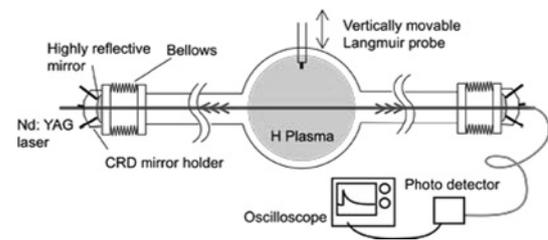
Fig. 1. Cross sectional view of the CRD system installed near the plasma grid in the FET-based ion source. The cavity length was  $\sim 1.3$  m and the plasma length was  $\sim 0.1$  m. Bellows were attached for mirror angle alignment.
