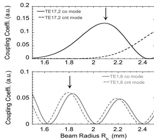
Fig. 1. Radial distribution of coupling coefficient of TE<sub>17,2</sub> and TE<sub>1,8</sub> modes. The solid line and dashed line stand for the co and counter rotating modes, respectively.
