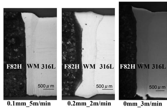
Fig. 1 SEM images of dissimilar joints between F82H and SUS316L produced by 4kW fiber laser.
