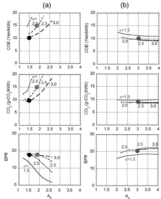
Fig.1. Cost of electricity (COE), CO<sub>2</sub> emission rate and energy payback ratio (EPR) for (a) ST and (b) TR designs as functions of plasma aspect ratio  $A_p$  and ellipticity  $\kappa$ . Solid circles denote three reference designs; ST-1A(black), ST-1B(green) and TR-1(red).
