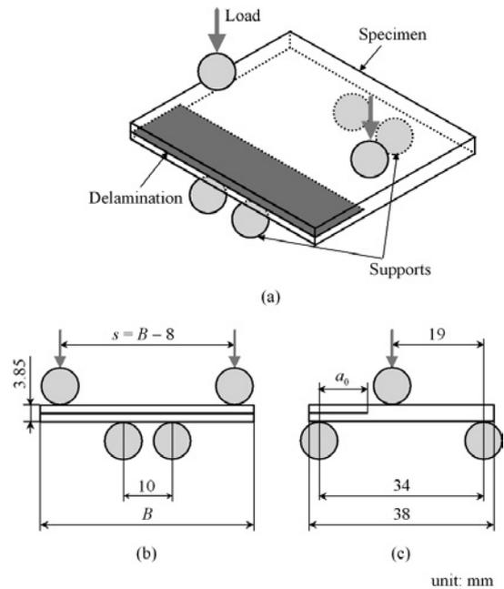
Fig. 1. (a) Perspective, (b) front and (c) side views of the 6PBP test setup.
