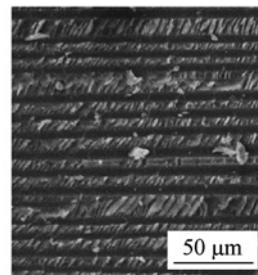
Fig. 2. Fracture surface at 4 K for  $G_{III}/G_T = 0.56$  (delamination growth from left to right).
