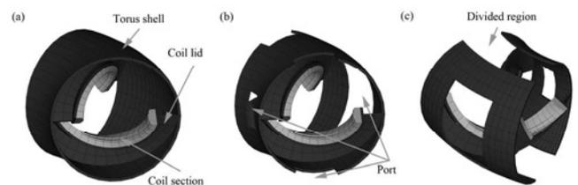
Fig. 3. 3-D FE models: (a) full torus shell, (b) torus shell with port, (c) widely divided shell.
