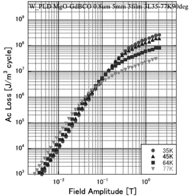
Fig. 1 Observed magnetic field amplitude dependences of the ac losses of the 5-filament GdBCO superconducting tape.
