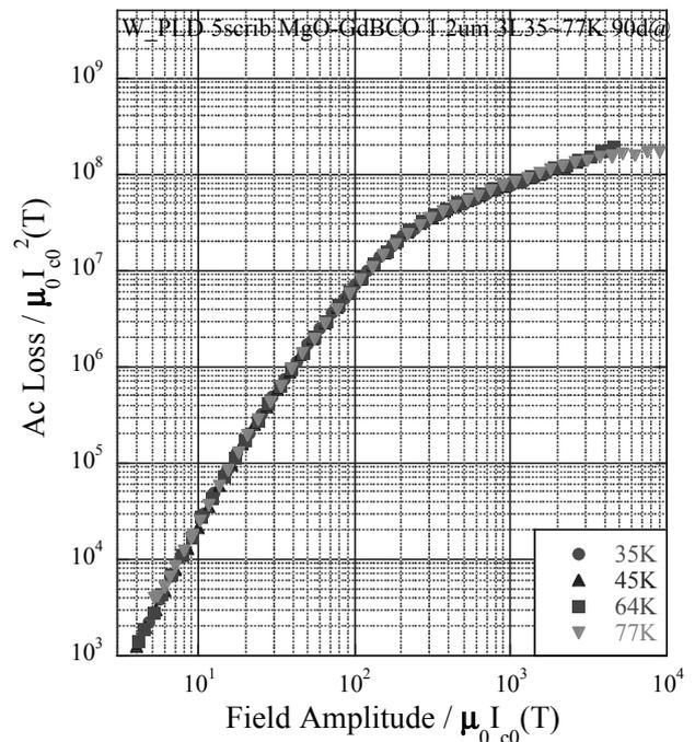
Fig. 2 Normalized magnetic field amplitude dependences of the ac losses of the 5-filament GdBCO superconducting tape.
