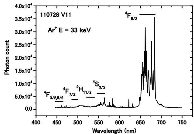
Fig. 2. Ion-beam induced luminescence spectrum in a visible range [4]. The spectrum was obtained using a grating of 300 Grooves/mm.
