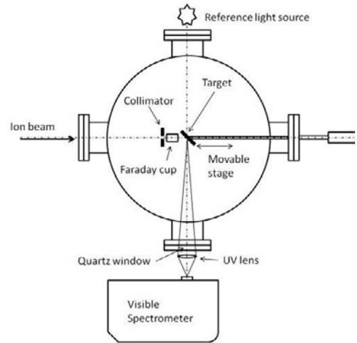
Fig. 1. Schematic illustration of the collision chamber and the visible spectrometer [4].
