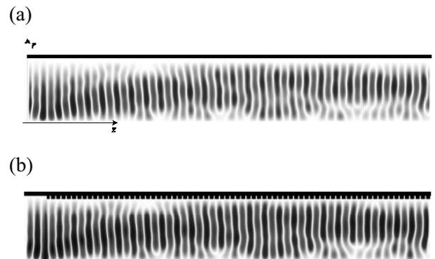
Fig. 1. The  $r$  component of magnetic field in  $(r, z)$  plane at time  $700 \times \Delta t$ . (a) The normal waveguide: (b) The corrugated wave guide.
