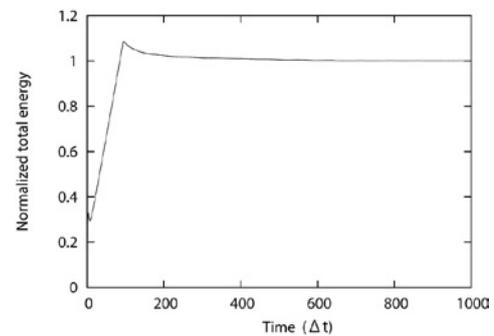
Fig. 2. Time dependence of the total energy for electromagnetic field in the corrugated waveguide. The energy is normalized by the saturated total energy.
