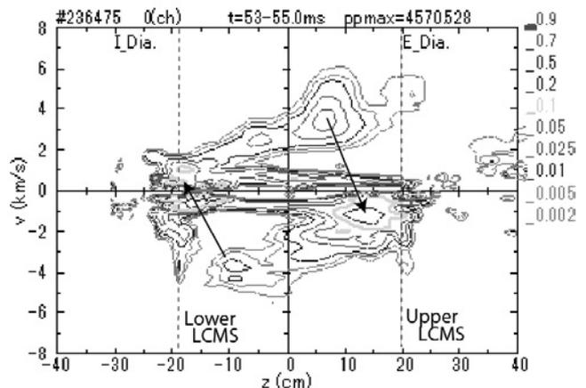
Fig.2 An example of the phase velocity of the measured density fluctuations. The phase velocity changed strongly near the LCMSs as shown by the arrows.
