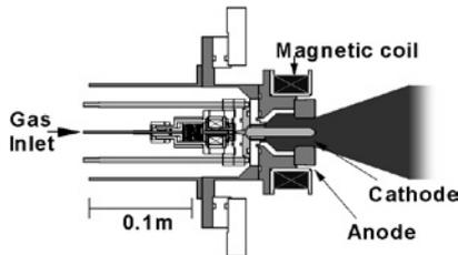
Fig. 1 Schematic of an MPD arcjet
