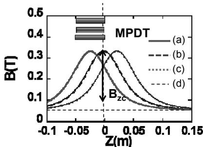
Fig. 2 Magnetic field profiles applied to the MPD outlet.
