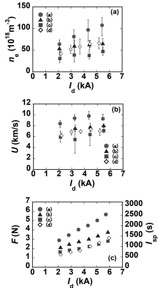
Fig. 3 Dependences of (a) $n_e$ , (b) $U$ , (c) $F$  and  $I_{sp}$  on discharge current  $I_d$ .
