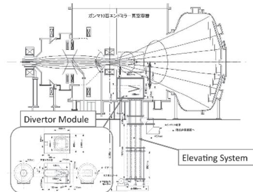
FIG. 1 The schematics of the new Divertor module installed on the west end section of the GAMMA 10 (PDX) for divertor plasma simulation experiment.
