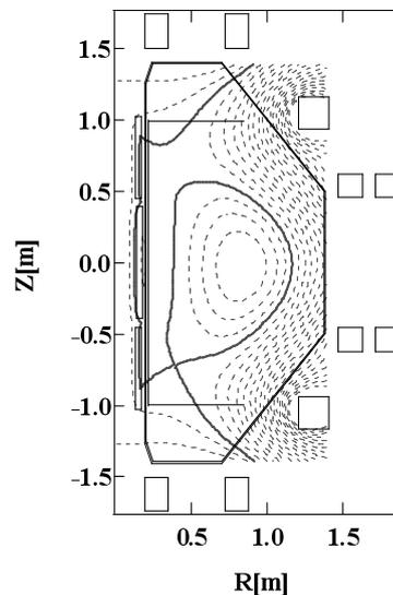
Fig. 2 Reconstructed magnetic surface structure in #13235 at 3.5s. The reconstruction was executed by parabolic current fitting (PCF) methods [1,3]. A lower single null configuration was achieved.
