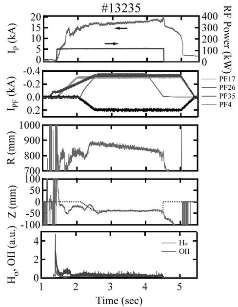
Fig. 1 Typical waveforms in a divertor configuration discharge are plotted. From top to bottom, panels display plasma current and injected RF power; currents applied to PF17, PF26, PF35, PF4 coils [1-3] dial position of the plasma; real vertical position (solid line) and destination (dotted line) of the plasma; and signals of  $H_{\alpha}$  and OII line radiation.
