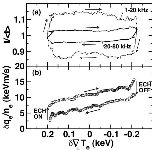
Fig.4 Non-linear electron-temperature gradient dependence of micro-fluctuation amplitudes and heat flux during ECH modulation. (a) Lissajous diagram of density fluctuation amplitudes and (b) gradient-flux relation. Arrows denote the direction of variation.
