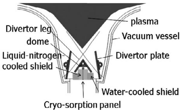
Fig.2 Horizontal cross-section of the equatorial plane of the closed helical divertor.
