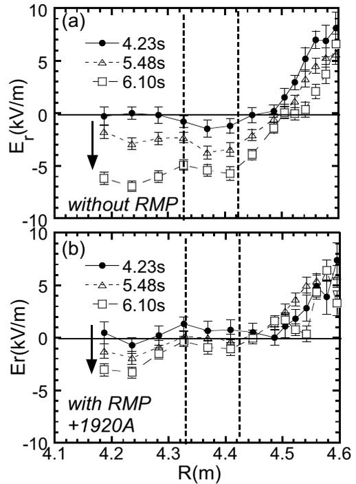
Fig.3 Radial profiles of radial electric field (a) without RMP and (b) with RMP in the discharges, where the direction of the NBI is switched from the co-direction to the counter-direction. Vertical dashed lines indicate the expected magnetic island by the RMP.
