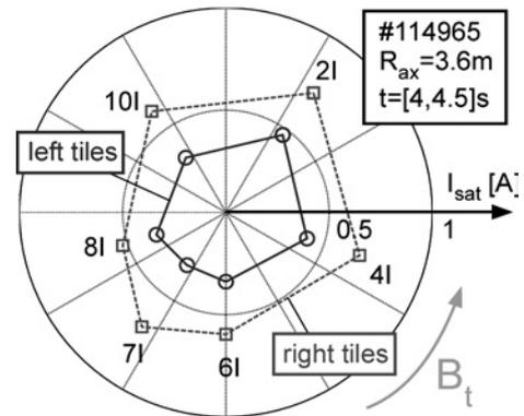
Fig. 2. Toroidal distributions of  $I_{sat}$  measured at left (blue line) and right tiles (green dashed line) during  $R_{ax} = 3.6$  m discharge with reversed  $B_t$ .
