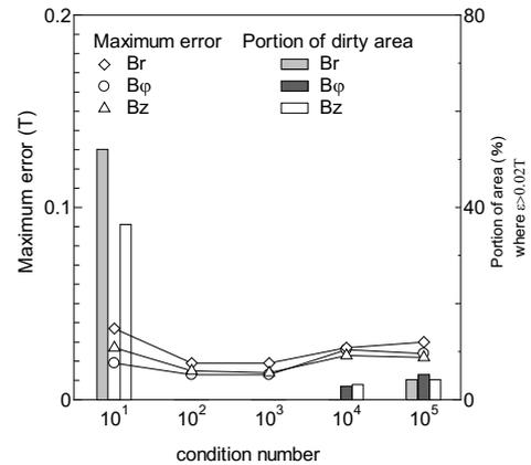
Fig.2 Error tendency of reconstructed field when assuming 440 field sensors and 126 flux loops with T8P6 boundary elements
