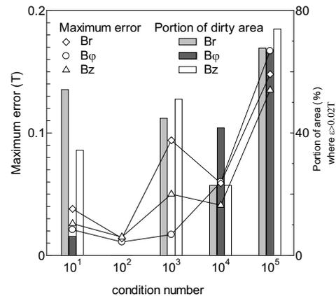
Fig.3 Error tendency when assuming a smaller number of sensors with T4P3 boundary elements
