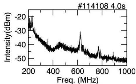
Fig. 4 Low frequency spectrum measured by discone antenna during EC wave injection.
