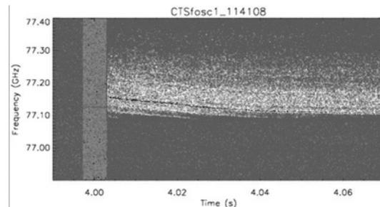
Fig. 3 High frequency spectrum measured by heterodyne radiometer during EC wave injection.
