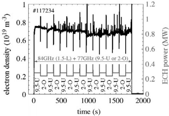
Fig. 1. Waveforms of the line average electron density (black) and the injection power of EC-waves (red) of the 30 min. discharge #117234.
