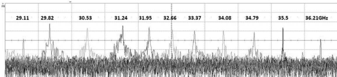
Fig. 1. Example of each frequency comb component reflected from corresponding cut-off layer in a LHD plasma. In this figure, the frequency spectra are over-plotted. The horizontal axis indicates the frequency (1MHz/div) and the vertical axis shows the power (10dB/div).
