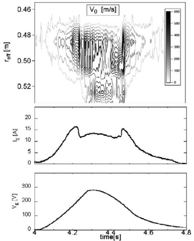
Fig. 2. Temporal behavior of radial profile of poloidal velocity (top: contour plot), current (middle), and bias voltage (bottom).
