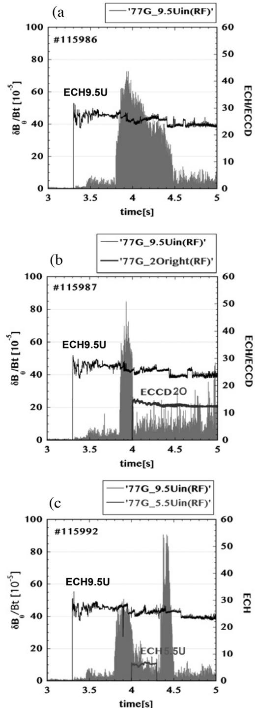
Fig. 1. Time evolution of  $n=1$  magnetic fluctuation amplitude, (a) without additional ECH/ECCD, (b) with counter-ECCD (20) and (c) with ECH (5.5U).
