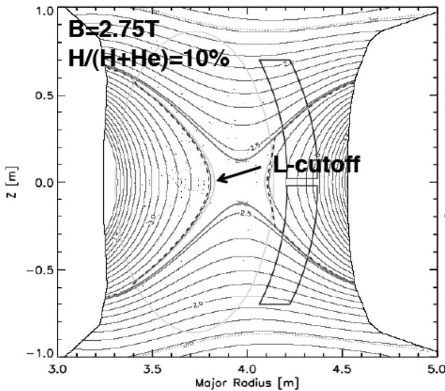
Fig.1 L-cutoff position on the contour map of the magnetic field strength at  $H/(H+He)=10\%$  in  $B=2.75\text{T}$ .
