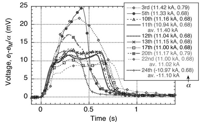
Fig. 3. Resistive components of normal zones that stopped within one pitch of the helical coil. The 3rd and 20th normal zones are considered to have propagated in the 2nd layer, and the others are in the 1st layer.
