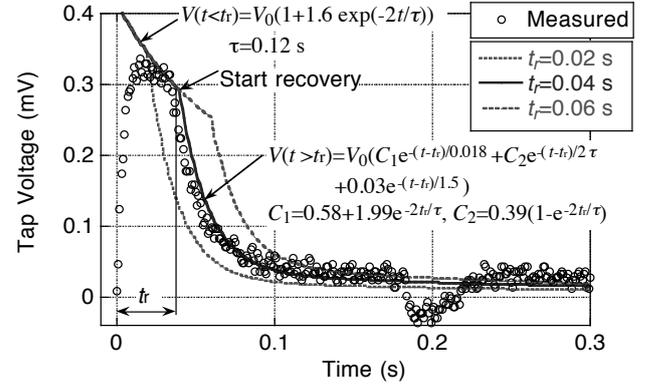
Fig. 1. Voltage drops of the LHD-HC conductor during propagation and recovery of a normal zone at 11.2 kA, 4.4 K. The distance of voltage taps is 23 mm.
