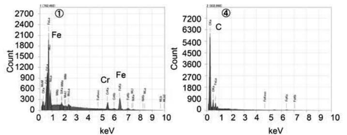
Fig. 3: EDS spectra at position ① and ④ in Fig. 1
