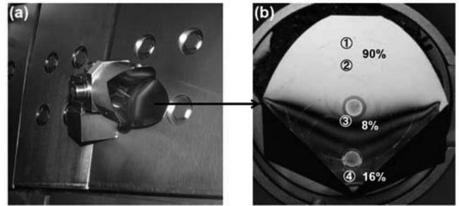
Fig. 1: (a) A retroreflector installed in LHD. (b) One of mirror pieces and the reflectivities at the visible laser light (633 nm). Circular marks near position ③ and ④ was made by GD-OES analyses (not discussed in this report).
