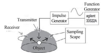
Fig. 1 Pulsed radar system
