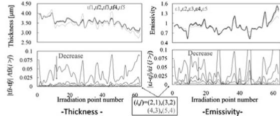
Fig.3 Distribution of foil thickness and estimated emissivity by the conventional method.
