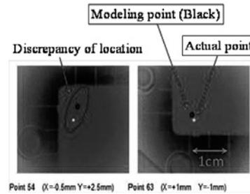
Fig.2 Photograph showing discrepancy of location.
